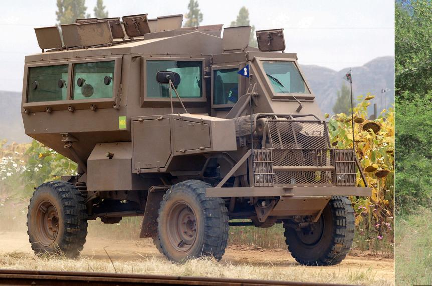
Fitted with an enclosed troop compartment the MK IIA Moffel is a mine resistant ambush protected troop carrier, locally built on a Unimog chassis
