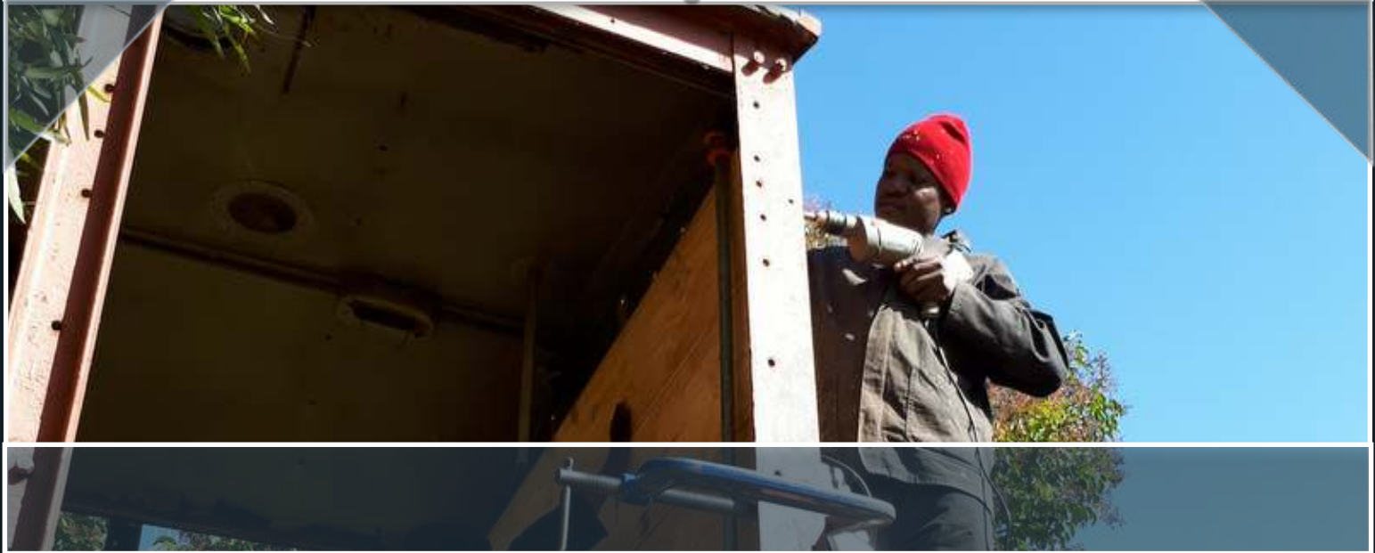
Ernest has now started to fit back the treated planks to the first 3'6" Goods wagon in Hoekfontein.
