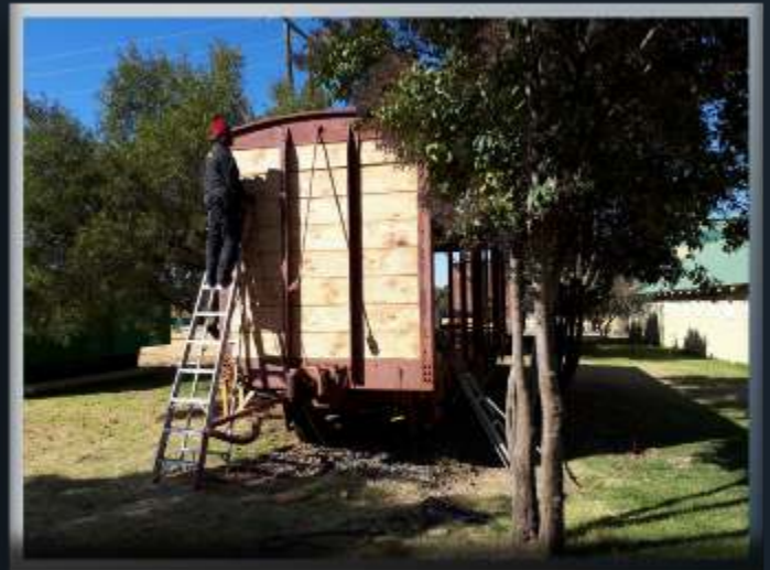
Ernest has now started to fit back the treated planks to the first 3'6" Goods wagon in Hoekfontein.
