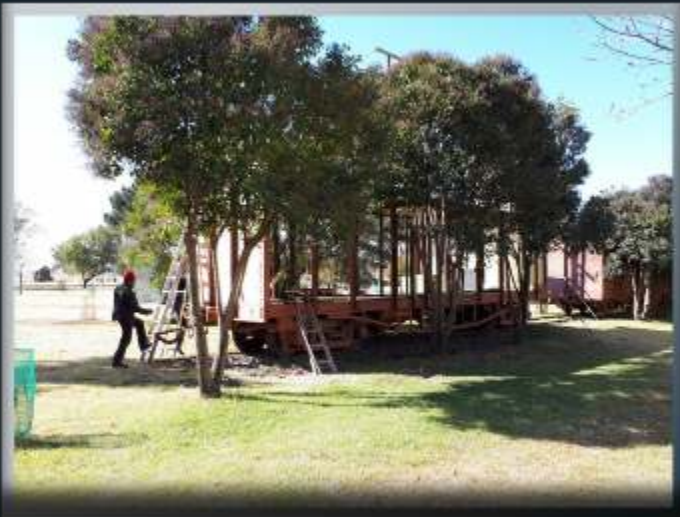
Ernest has now started to fit back the treated planks to the first 3'6" Goods wagon in Hoekfontein.
